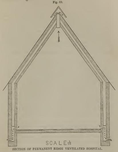
I cannot conceive of a more efficient system, both of heating and ventilating, than this, nor one which is more simple in its operation. In apartments in which it is impossible to secure ridge ventilation, a great deal can be done by the construction of flues, by which the foul air is removed from the room. One of the best of these, and one which can readily be adapted to permanent buildings, is that of Dr. Arnott, and which is shown in Fig. 70.
